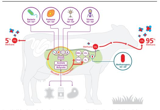
Notes: Microbial numbers are listed per ml or gram of ruminal contents. Abbreviations:  $CO_2$  = carbon dioxide;  $H_2$  = hydrogen,  $CHO_2$ ? = formate;  $CH_3X$  = methoxy compounds or methylamines;  $CH_4$  = methane. Source: Image courtesy of the New Zealand Agricultural Greenhouse Gas Research Centre (www.nzagrc.org.nz).
